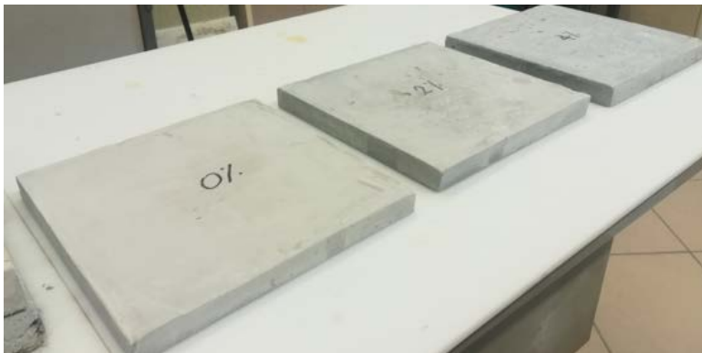
Fig.7. Images of blocks of cement for analysis of thermal conductivity
